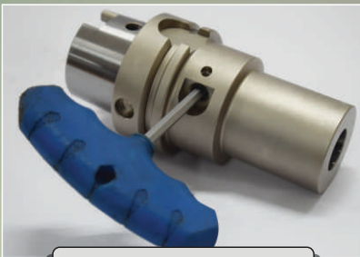
Extremely fast tool changing with a turn of 'T' wrench
